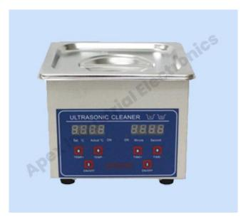
Ultrasonics (Ultrasound) is the sound which human beings cannot hear. Ultrasound utilizes frequencies of 40 kHz. High frequency electrical energy is converted into ultrasound waves by means of ultrasonic Transducers, which are bonded on the base of S. Cleaning Tank. These high frequency sound waves create in the liquid countless, Microscopic vacuum Bubbles which rapidly expand and collapse.
